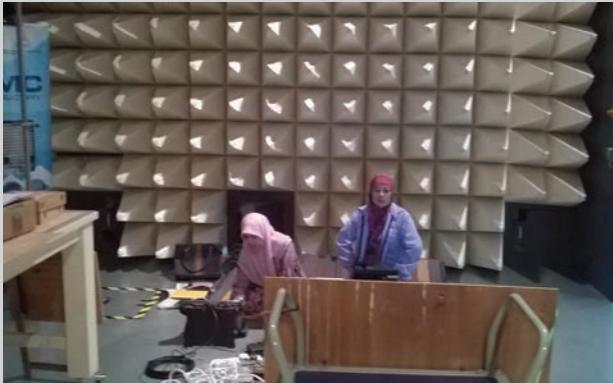
Pengujian kesan GPS antenna orientation
